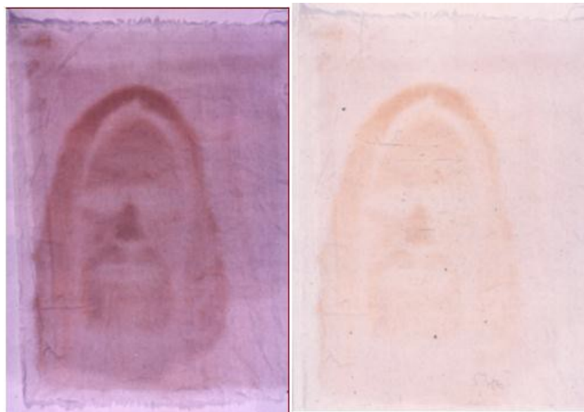
10/ On the left: a positive photograph of the test piece of linen (previously prepared with dilute silver nitrate) showing the negative image produced after three days. This image is a composite of oxidised lined and silver atoms. On the right, the same negative image after all silver nitrate has been removed with ammonium hydroxide. (c. 1992). The image on the right is only formed by oxidised fibrils on the surface layers of the linen. Any silver atoms still present will be parts per million at best. (Copyright: Mr Glenn Meyer)
