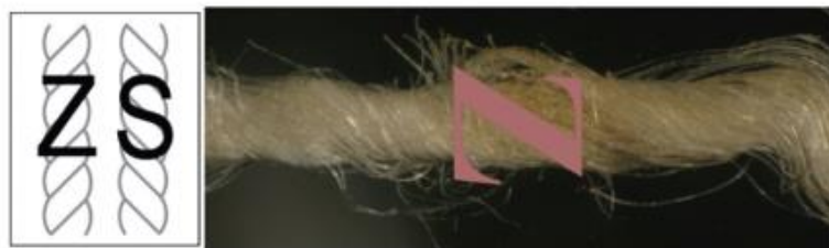
Figure 5.6 On the left: Schematic drawing of the “Z” twist and the “S” twist yarn. On the right: Magnification of the Shroud cloth of Fig. 1.5 in which we clearly see the clockwise twisting (“Z” twist) of the flax fibers into yarn.
