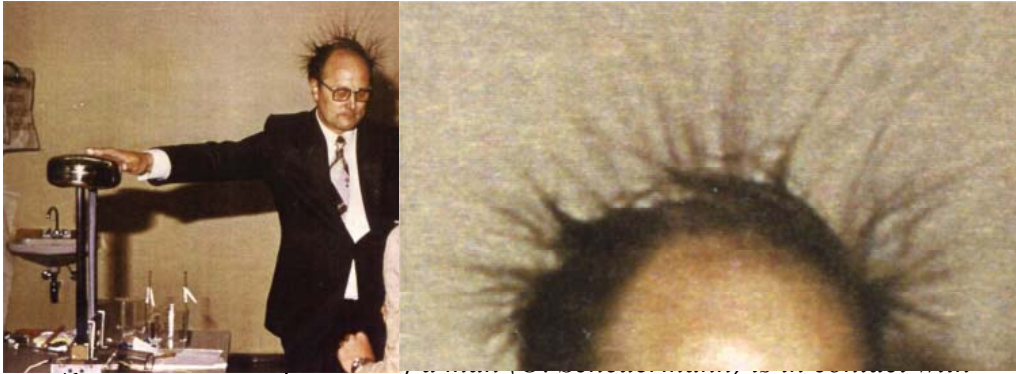
the high-voltage electrostatic field produced by a Van de Graaff generator.
