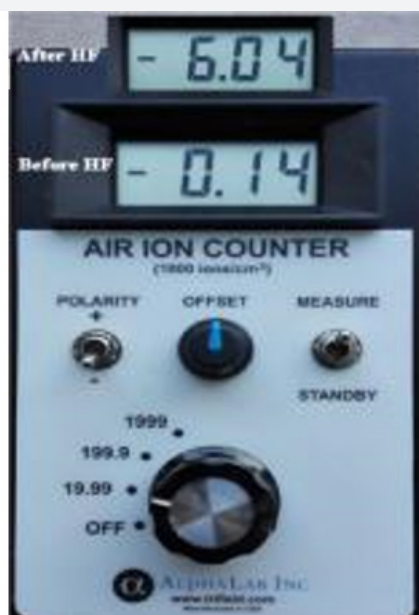
Figure 12: The air ion counter measured 140 negative ions/cm 2 before the HF ignition, while during the HF the reading raised up to 6040 negative ions/cm 2 .
