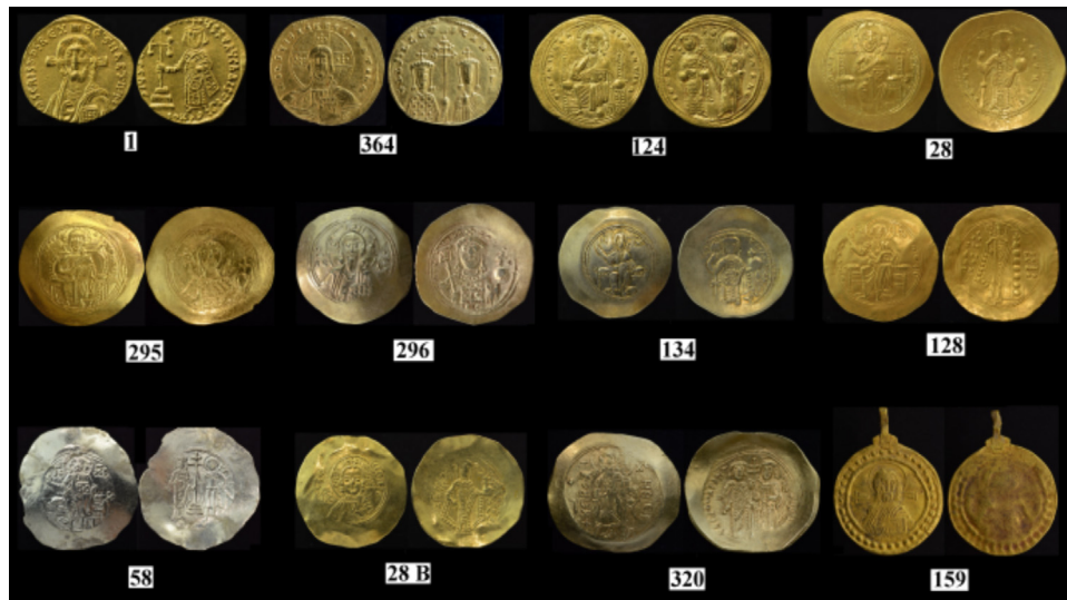
Fig. 2. Example of the set of coins and medal tested with EDX.
